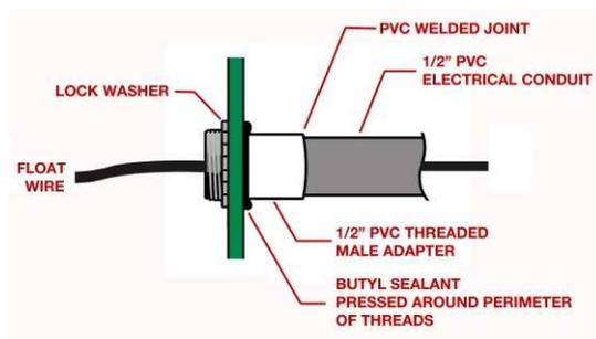
Caulk around cable in conduit to block septic air flow to control panel.
