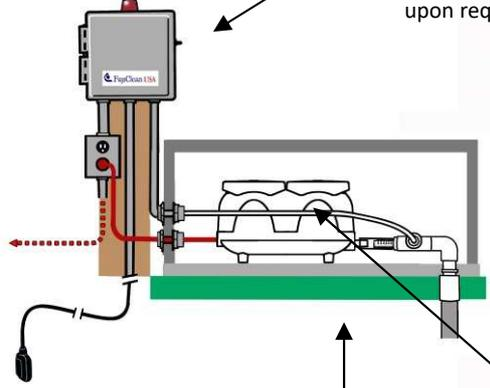
FujiMAC "RII" Commercial Series linear diaphragm air pump, typically 150-300 liters/min for commercial applications.
