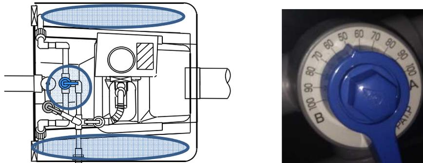
□ **9. Check/Set Effluent Airlift Valve (white).**
