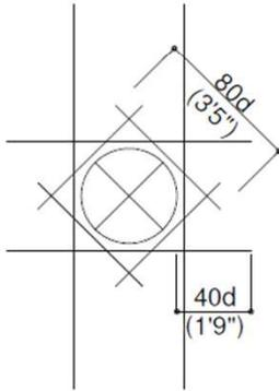
d : DIAMETER OF FERRO REINFORCEMENT MATERIAL
