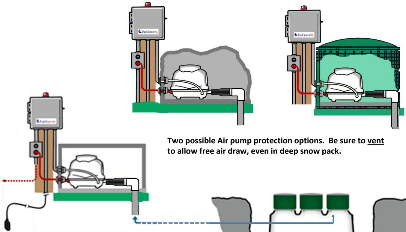
Two possible Air pump protection options. Be sure to vent to allow free air draw, even in deep snow pack.
