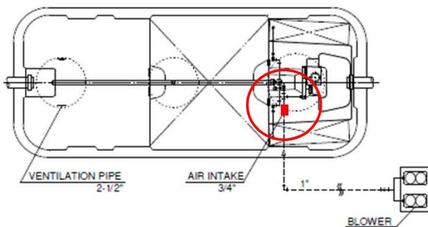
For connection air line to tank, use approved sealant to prevent septic gas transmission into control panel.
