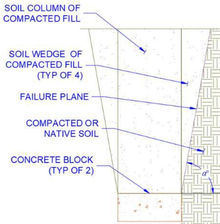
**Figure 8 - Soil Wedge Approach for Uplift Restraint**
