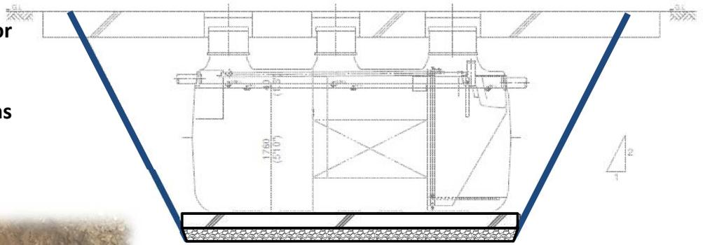
Check that concrete is level to 1/8" per 2 feet (10mm per 2 meter or 1/200), (fore and aft as well as side to side).
