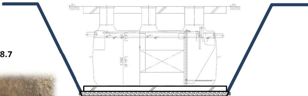
Check the concrete is level to 1/8" per 2 feet (10mm per 2 meter or 1/200), (fore and aft as well as side to side).
