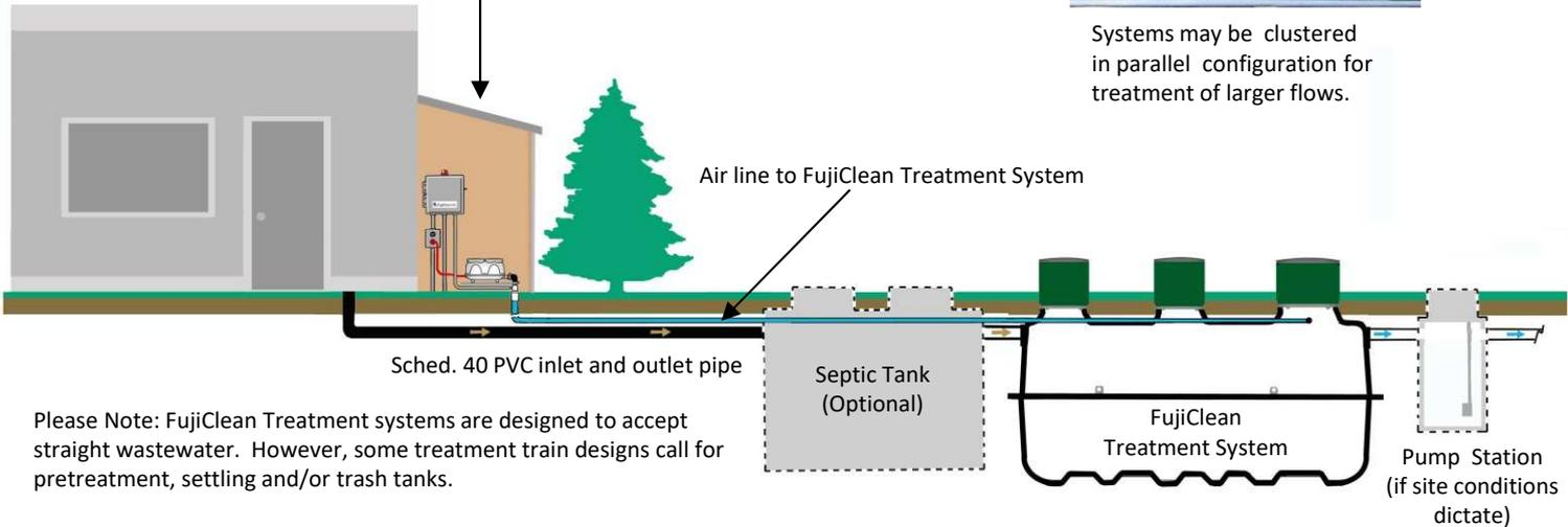
Please Note: FujiClean Treatment systems are designed to accept straight wastewater. However, some treatment train designs call for pretreatment, settling and/or trash tanks.
