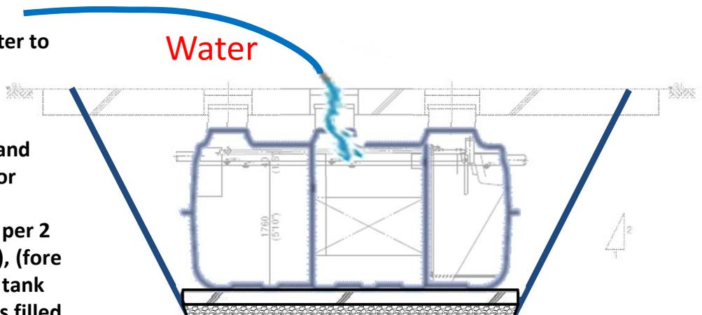
To ensure tank water tightness, check in 24 hours to be sure that the water level has not dropped. Contact your distributor or FujiClean USA if water level has dropped.
