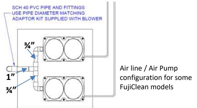
Note: Air pump connection piping does not count toward "5-elbow" limit
