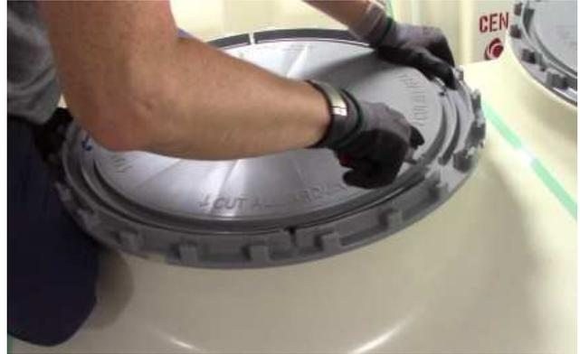
Use sharp blade to remove inner plastic ring.
